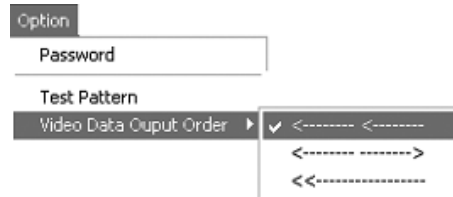
FIGURE 32. Use the “Option” menu to access the test pattern.
